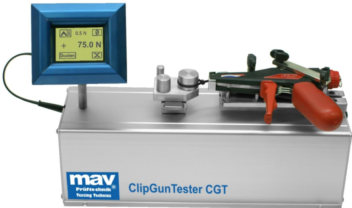
Clip Gun Tester CGT 50 with KBP toolset and HellermannTyton cable tie tighten pistol MK 7
