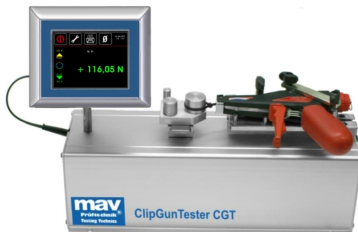
Tool Set KBP-MK 9 on a Clip Gun Tester CGT
