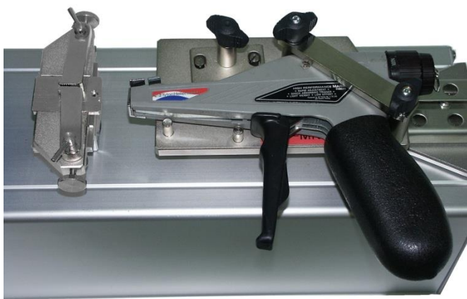
HellermannTyton MK 7 with CGT 50 and quick action clamp KSH 6
