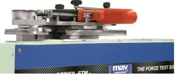
The KBP-A tool enables a continuous testing due to the electromotive drive of the machine's load sled. The options force preset, movement path preset and testing speed preset can be chosen and adjusted.
