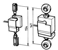
Load Cell 50 to 1000 N with fork heads M6 Load Cell 2000 to 10000 N with ball screws M12
